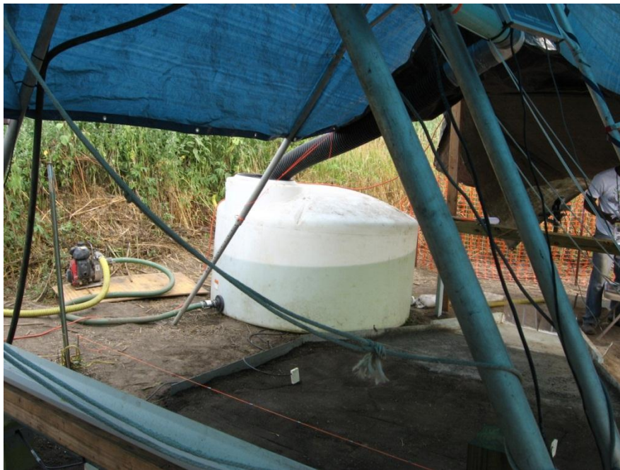
Figure 5.4 Water tanks used to store the excess water from the return pipe in the rainfall simulator.
