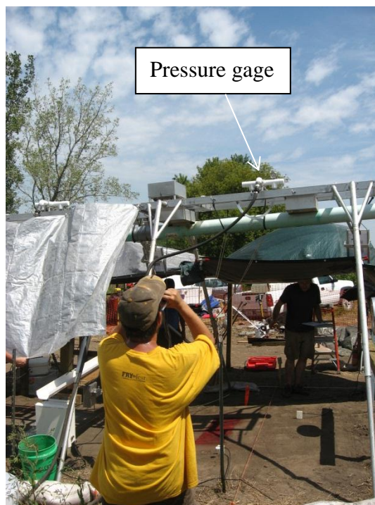
Figure 5.5 Checking the pressure in the pipes during the experiment using binoculars.
