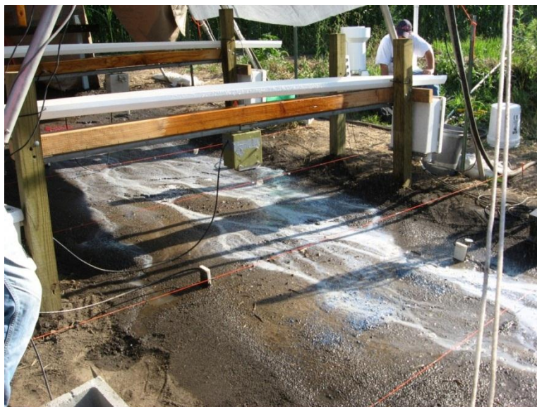
Figure 5.31 Milk dye tracer applied during the progression of the experiment.
