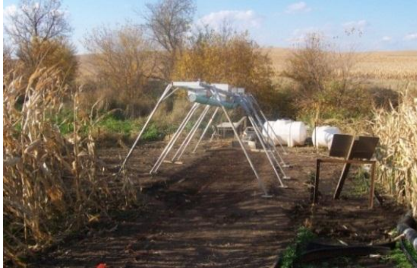
Figure 5.3 The 3 rainfall simulators placed in series located in the experimental station.
