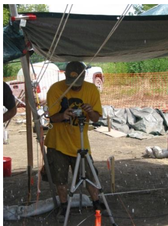
Figure 5.18 Video recording of the experiments via a video-camera placed at the plot outlet.
